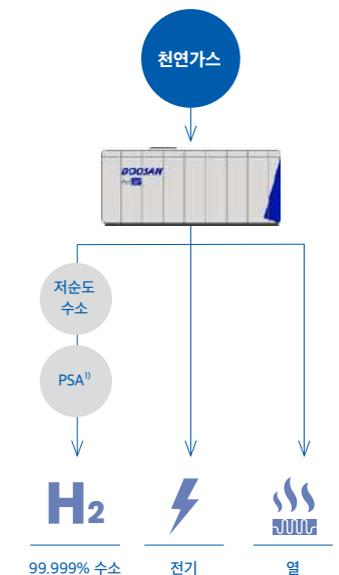
1) PSA: Pressure Swing Adsorption
